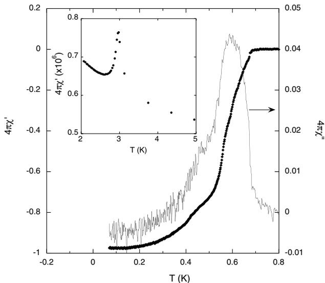
FIG. 2. Real and imaginary components of the ac susceptibility as a function of temperature in a zero applied field. The probe field was 0.05 G. Note that a full Meissner state is formed below  $\sim 0.3$  K. Inset: ac susceptibility as a function of temperature showing an antiferromagnetic transition at  $T_N = 2.97$  K.
