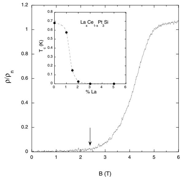
FIG. 5. Transport critical field transition in CePt<sub>3</sub>Si at  $T = 70 \text{ mK}$ . The arrow depicts the field above which there is no longer a diamagnetic response in the susceptibility. Note that this is also approximately the field at which the onset of resistance occurs. Inset: transition temperature of  $\text{Ce}_{1-x}\text{La}_x\text{Pt}_3\text{Si}$  as a function of  $x$ .
