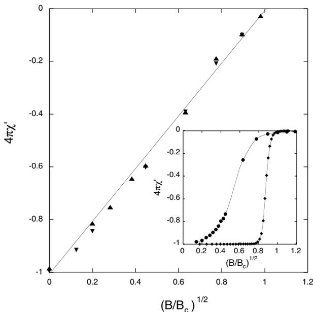
FIG. 4. Square-root field dependence of the susceptibility of two CePt<sub>3</sub>Si samples at 70 mK. The line is provided as a guide to the eye. Inset: the circles represent the 10 K susceptibility of the noncentrosymmetric A15 superconductor V<sub>3</sub>Si. The diamonds are data from a Pb sample alloyed with 5% Sn in order to make it type II. Note that neither of these latter systems obey a square-root scaling law.
