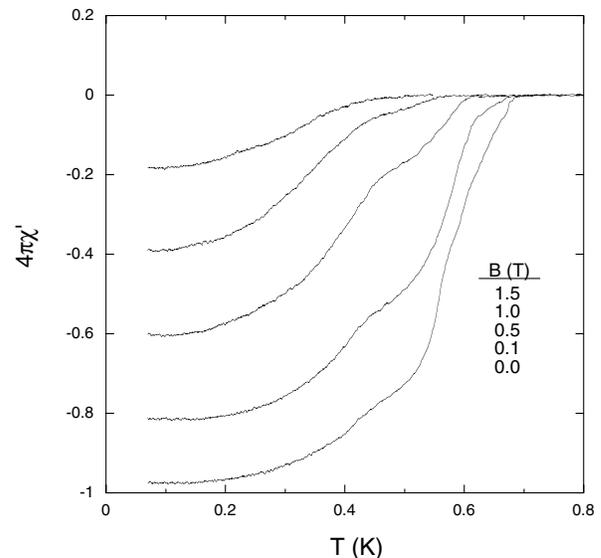
FIG. 3. Susceptibility as a function of temperature in an external magnetic field. Note the rapid increase in  $4\pi\chi'$  upon the application of relatively modest fields. The field at which the diamagnetic response was completely attenuated was  $B_c \sim 2.4$  T.
