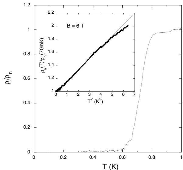
FIG. 1. Relative resistivity of CePt<sub>3</sub>Si as a function of temperature. The midpoint of the superconducting transition is at  $T_c = 0.72$  K. Inset: quadratic temperature dependence of the normal state resistivity.
